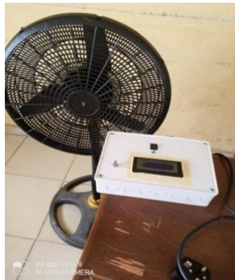
Plate 3: The constructed automatic fan regulator using Bluetooth.
