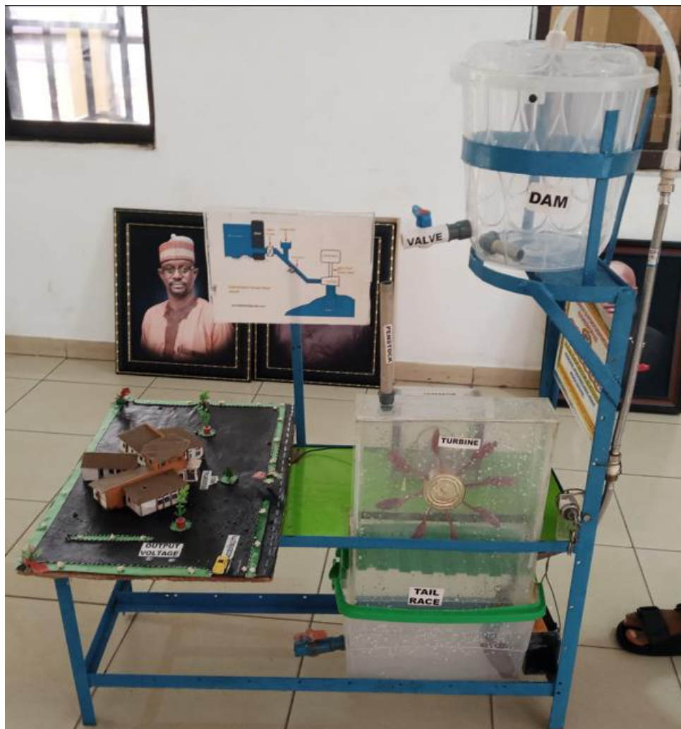
Fig. 5: Hydropower turbine model constructed at Federal Polytechnic Idah, Nigeria
