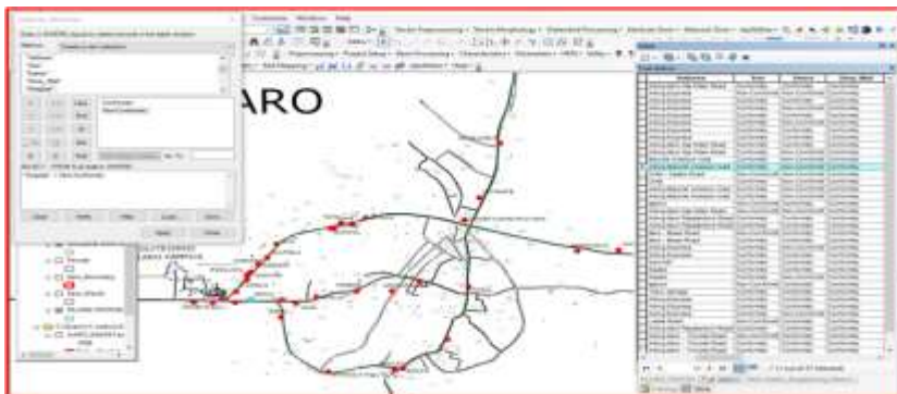
Figure 10: Query result of Filling stations whose 100m setbacks from Hospitals are not in conformity with planning standards.
