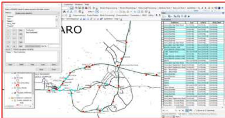
Figure 9: Query result of Filling stations whose 100m setbacks from Eateries are not in conformity with planning standards
