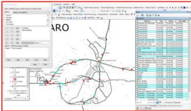
Figure 8: Query result of Filling stations whose 400m radius from the nearest neighbor filling station on either side of the road are not in conformity with planning standards.
