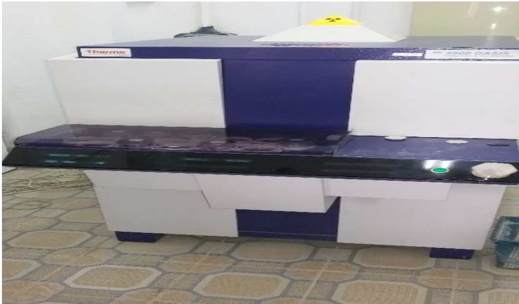
Figure 2: XRF machine at Quality Control Laboratory of Lafarge cement factory at Ewekoro
